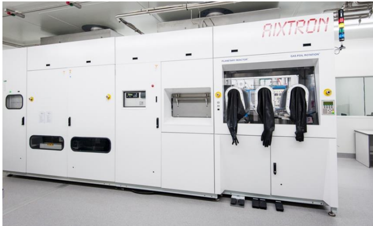
The AIXTRON G4 system being retrofitted onsite at BluGlass
